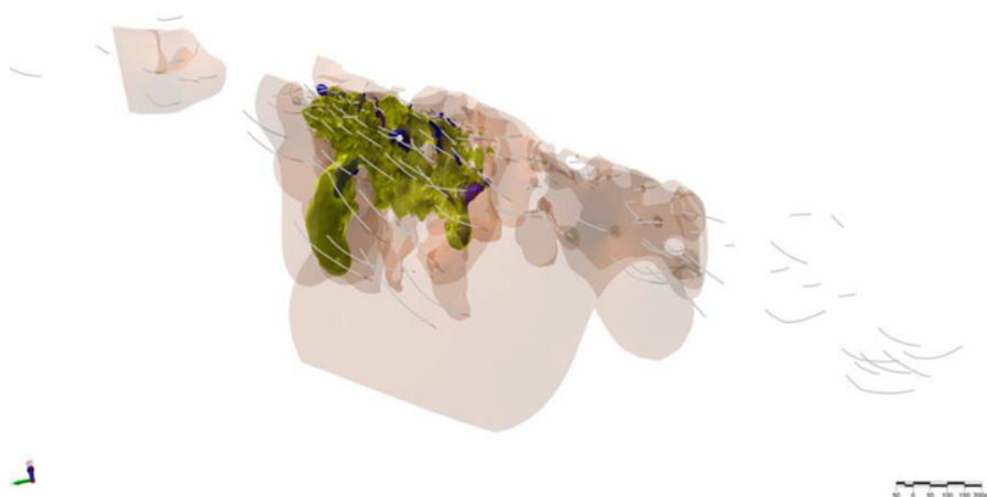
Figure 16: Extensive wireframed domain for copper (transparent orange), in comparison to the wireframed regions of gold (yellow) and silver (blue), showing their relative limited spatial distribution compared to copper, within the mineralized zone
